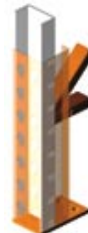
Rollformed "C" Insert (cut away view)
