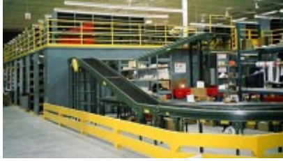
Mezzanine with Conveyor
